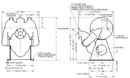
3" FLANGED SUCTION & DISCHARGE • 34" NPT AIR INLET PORT • 1" NPT AIR EXHAUST PORT
